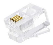
**Avalon** RJ11 Cat.3 Connectors are designed for today's high performance networks. A superior two-prong contact design works for both Solid and Stranded conductors. An integrated strain relief boot holds the cable in the proper position while crimping and provides protection to the cable connection after installation.
