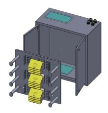
Avalon Mini ODF / Wall Mount Fiber Splice Enclosure can support up to maximum 288 splicing with 24 splice trays which support 12 splicing per tray. It is designed to install in building entrance or data centers and Floor Telecom facilities / closets for cross-connection between the distribution cables and drop cables.
