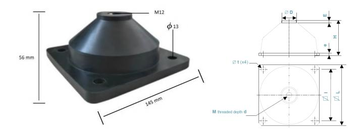
Avalon's multi-directional Anti-Vibration Shock Mounts, these isolators include great features, such as their wide temperature range, high adaptability and resonance frequency up to 14 Hz and are suitable for static loading per mount of 30 to 1,200 Kg
